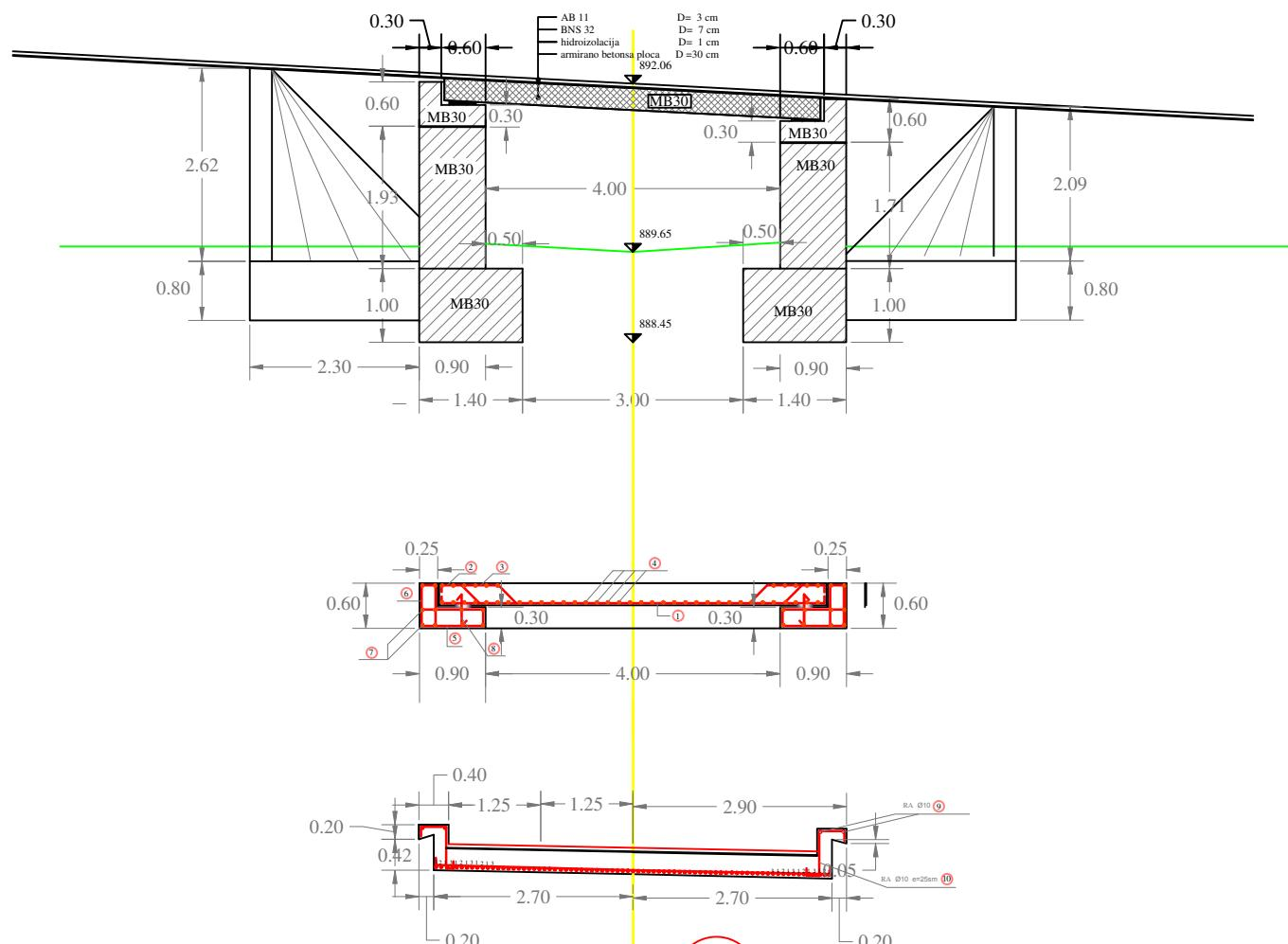
SPECIFIKACIJA ARMATURE ZA PLOČAST PROPUST
