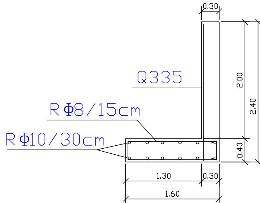
SPECIFIKACIJA ARMATURE AB PÖTPÖRNI ZID L=10M, h=1.5M
