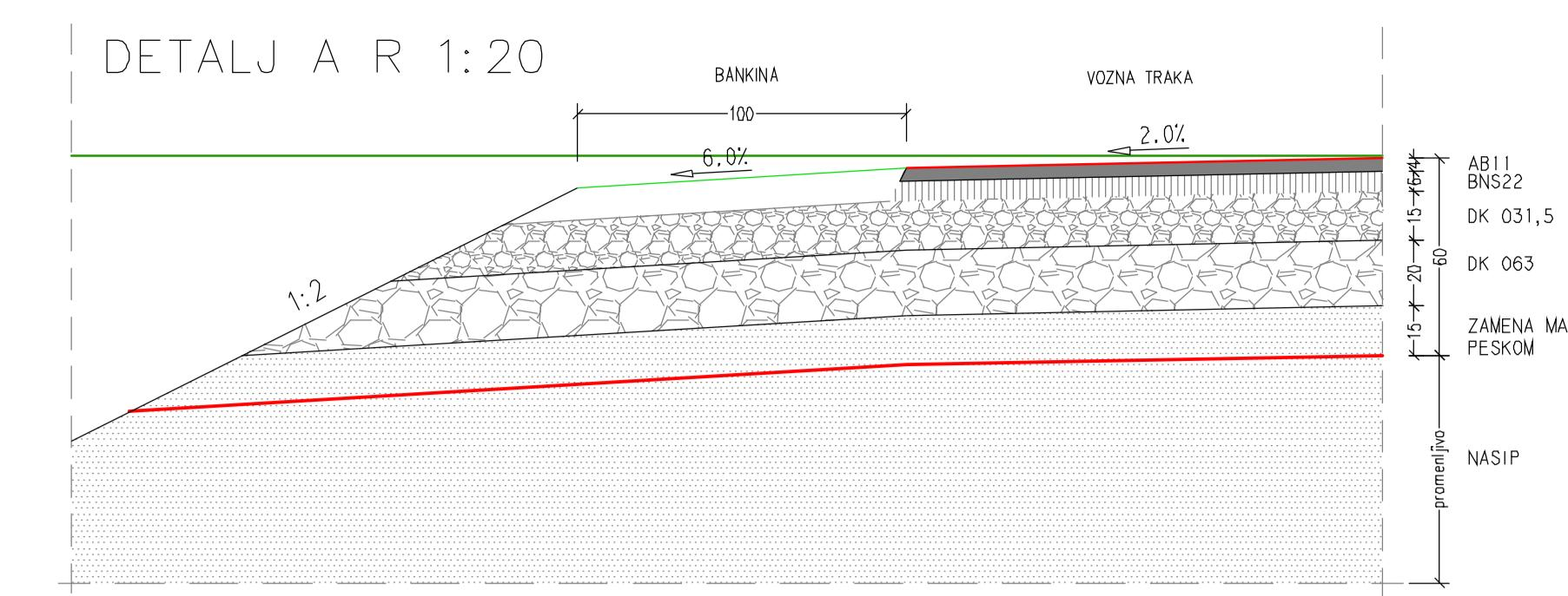
NORMALNI POPREČNI PROFIL NA MESTU MIMOILAZNICE R 1:50
